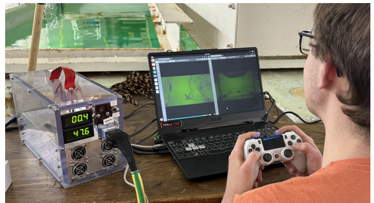
Figure 13: Topsides Control Station, Credit: Mark Johnson, 2026
