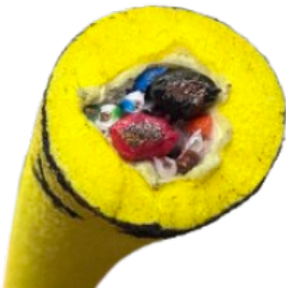
Figure 9: BlueStar's Tether Cross-Section, Credit: Mark Johnson, 2026
